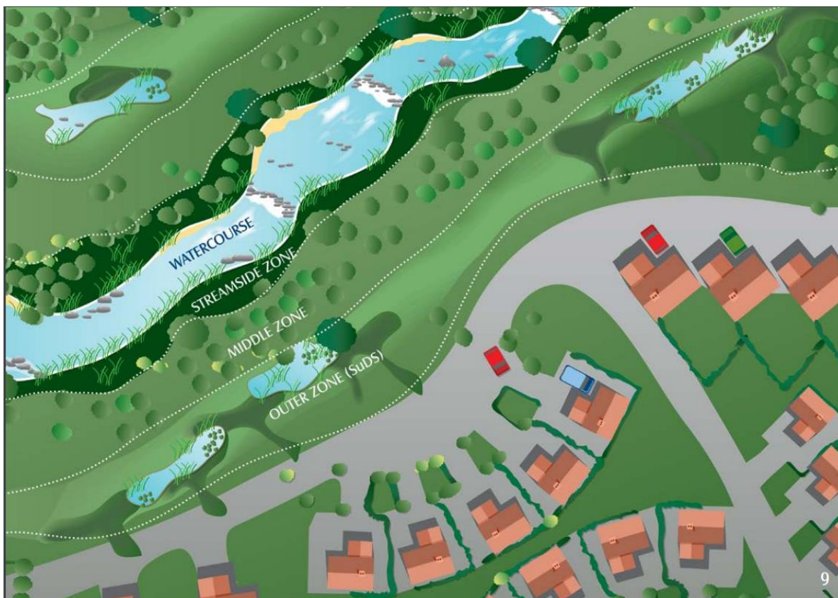
Figure 4.1: Riparian Zones for Urban Areas (IFI - Planning For Watercourses In The Urban Environment)
